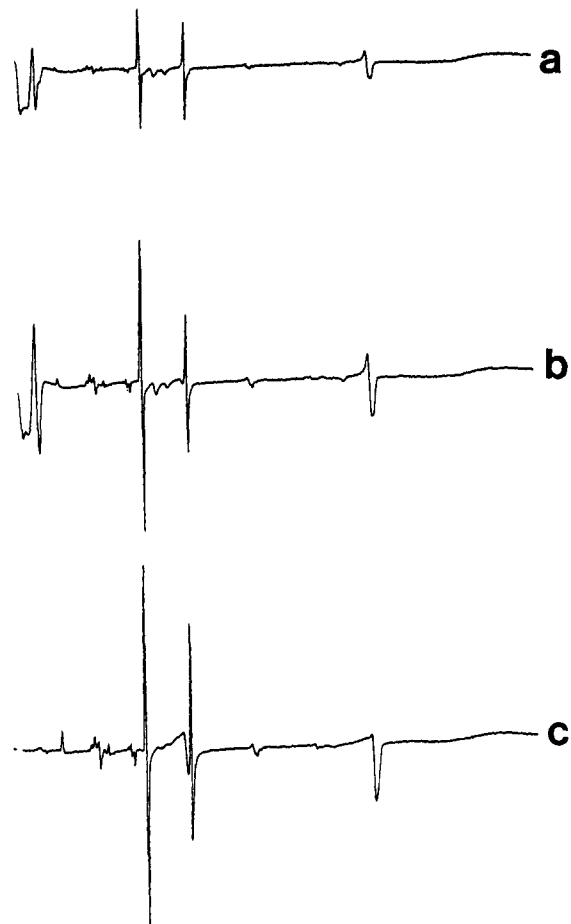
Figure 4. ESR spectra at different temperatures from photolysis of a single sample of 9 in 2-MeTHF. \nu_0 = 9.34 GHz, 100–9800 G. Temperatures: (a) 60 K, (b) 22 K, (c) 5 K. The same ordinate scale is used for curves a–c, so the relative peak intensities are properly displayed.
